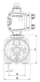
Height with controller fitted H3 + approx 226mm = 370mm
